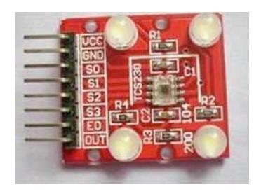
This Color Sensor is a complete color detector, including a TCS230 RGB sensor chip and 4 white LEDs. The TCS230 can detect and measure a nearly limitless range of visible colors.
