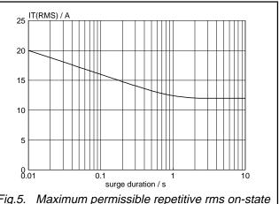
Fig.5. Maximum permissible repetitive rms on-state current  $I_{T(RMS)}$ , versus surge duration, for sinusoidal currents, f = 50 Hz;  $T_{mb} \le 109$ °C.
